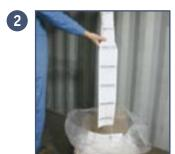
Unfold the ABSORBAG\*. Note: if the ABSORBAG\* is individually lined, cut open the liner bag. If the box is bulk lined for 12 AB-SORBAGS and not all are used, remember to re-close the liner bag in the box.
